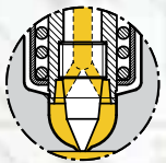
Pinpoint Style Tips (Standard & Wear Resistant)
